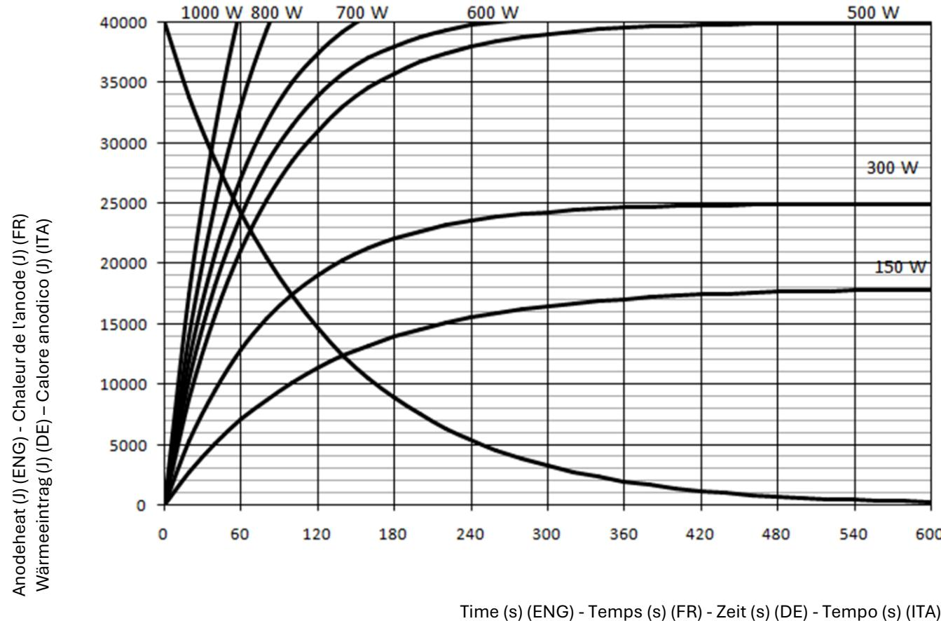
FILAMENT CHARACTERISTICS (ENG) - CARACTÉRISTIQUES DU FILAMENT (FR) HEIZWANDEL
